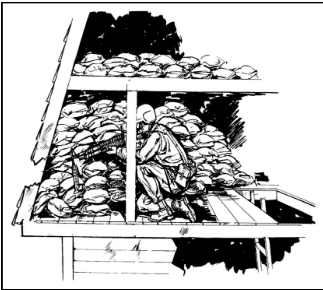
Figure 3-60. Firing platform built under roof.
